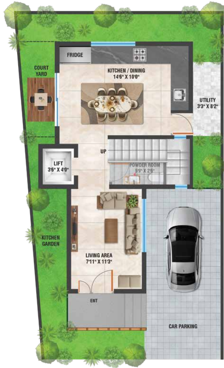
WEST FACING - GROUND FLOOR PLAN 7.1M X 11.9M [23'3" X 29'1"] BUILT UP - 494 SQ. FT.
